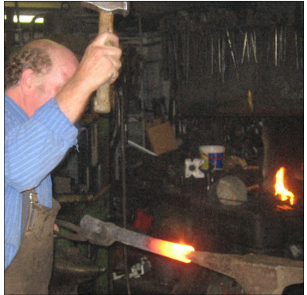
Fig. 13: The socket then is thinned out lengthened here on the horn.
