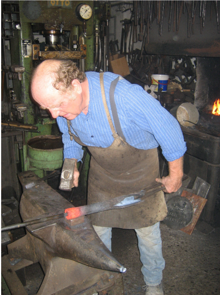
Fig. 7: Shaping the breech end of the future barrel. Note the inserted rod for keeping the bore open
