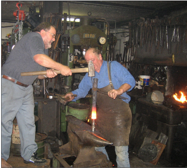
Fig. 12: The socket for stocking the finished gonne and is widened up by hammering the rear end of the barrel over a thorn.
