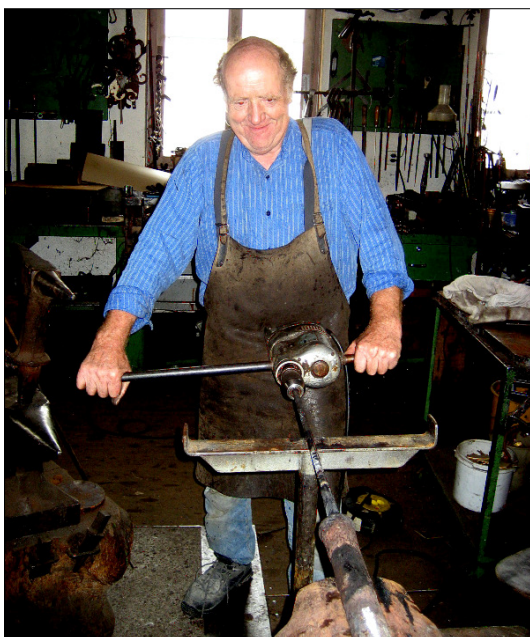
Fig. 14: Finally a breech plug is inserted and the barrel constricted behind it.
