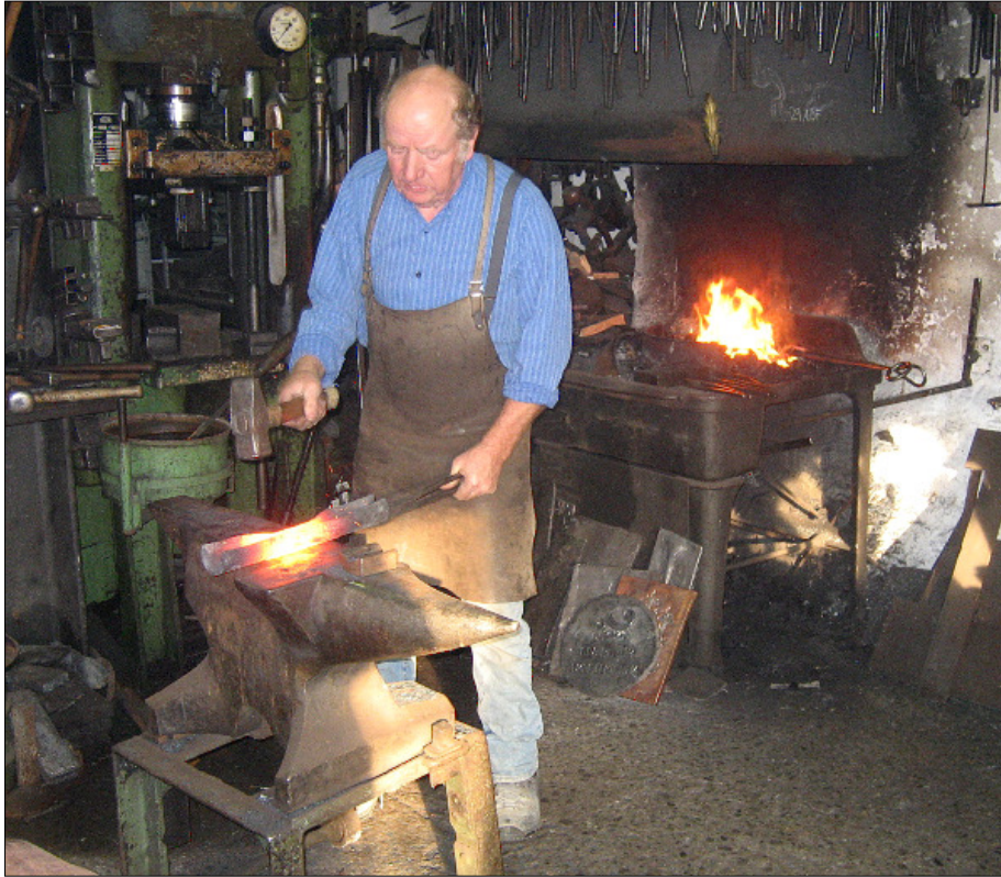
Fig. 5: Then the "U" is closed to form a pipe, starting in the middle of the pipe.
