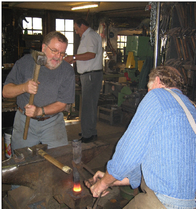
Fig 10: The muzzle cone is upset by hammering the finished pipe head-on vertically into a matching mould.
