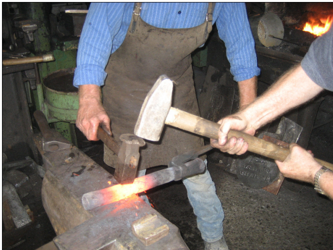
Fig. 14: Finally a breech plug is inserted and the barrel constricted behind it.
