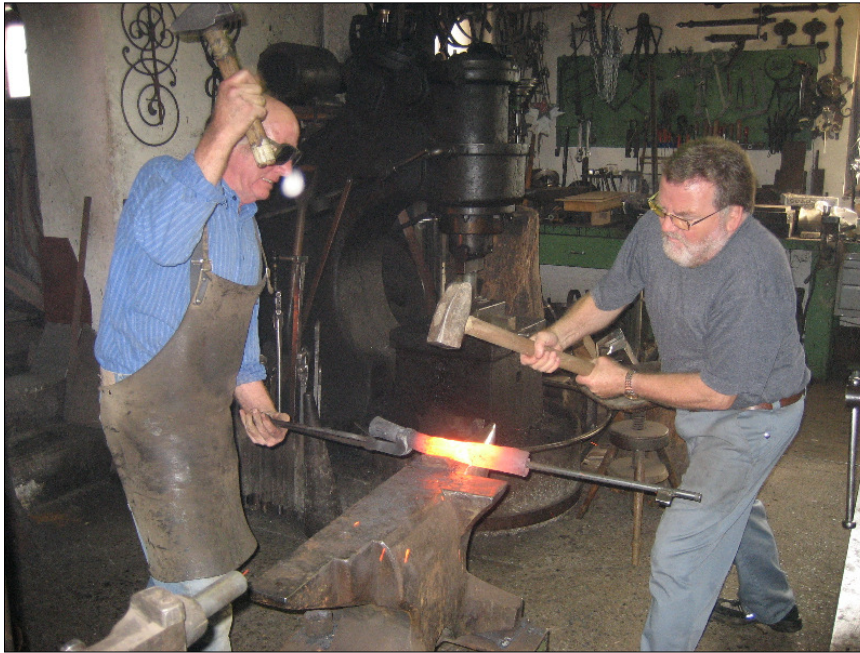
Fig. 9: Fire-welding. The two brothers quickly hammering the white-hot pipe. As flux a mixture of clay and glass powder is used. (Borax wasn't discovered then)
