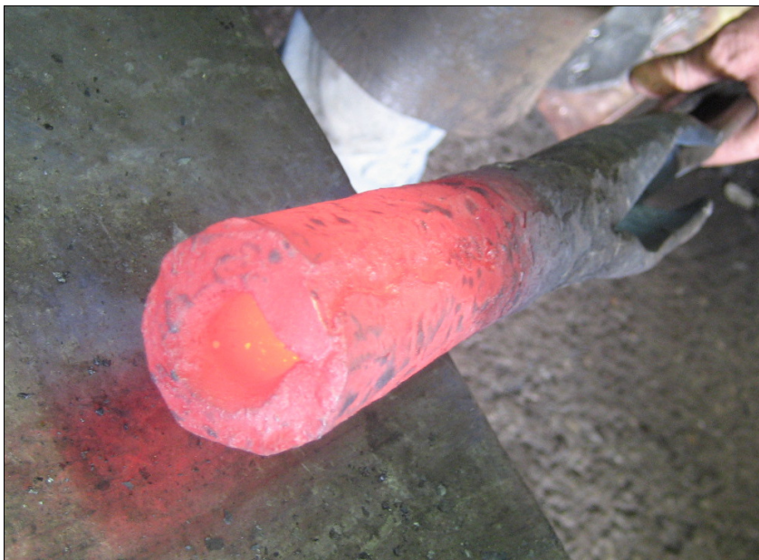
Fig 8: The overlapping seam of the rolled barrel.
