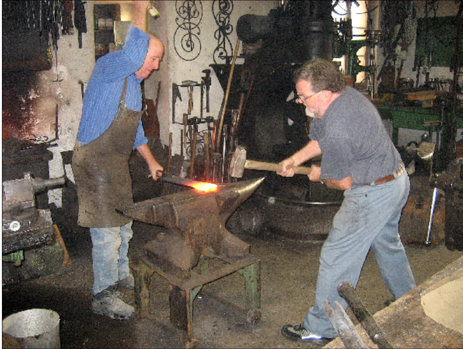
Fig 3: Benno, left, with his brother Otto bevelling the edges alongside of the flat iron bar as a first step. Note a finished Tabor handgonne laying on the table in the foreground.
