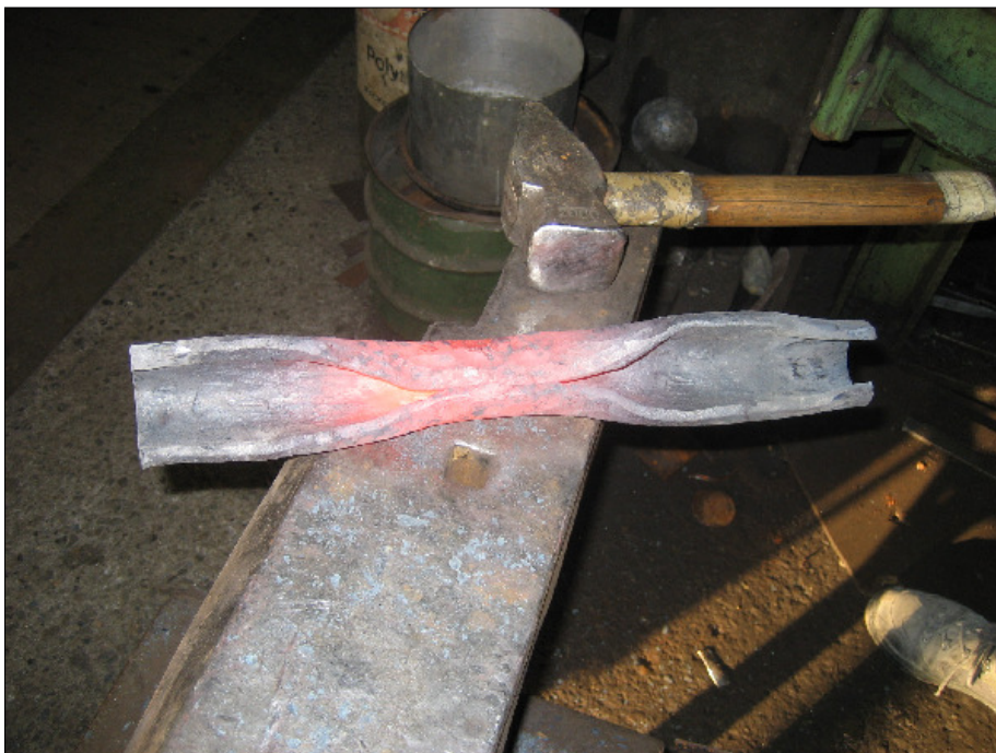
Fig 6: This is the first step of rolling the "U" to a pipe.
