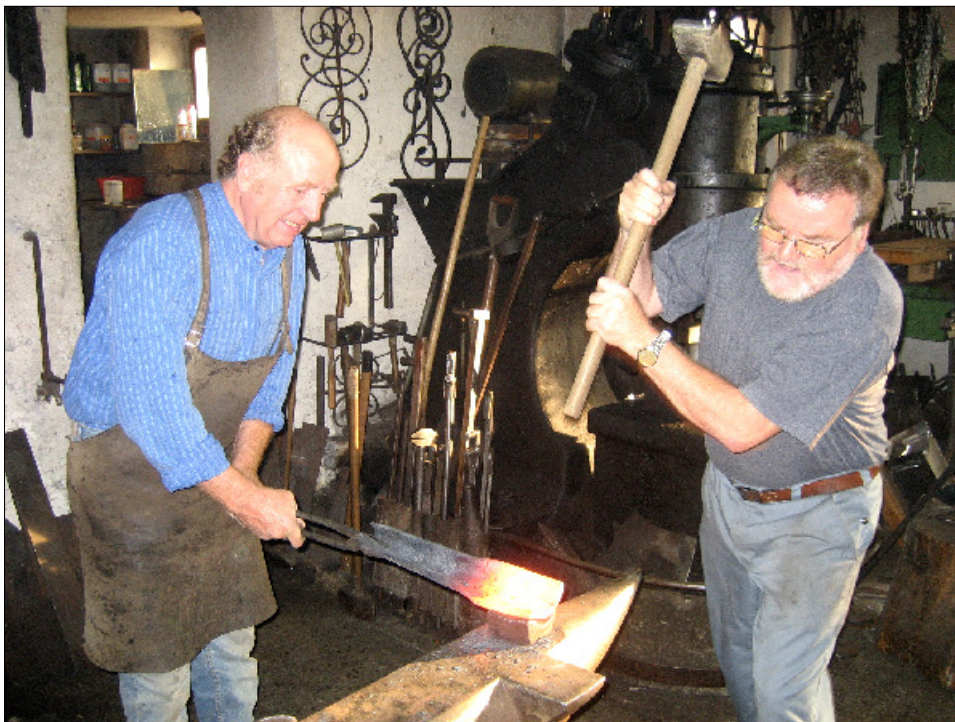
Fig. 4: Here the flat bar is bent to U-shape, hammering it into a mould.
